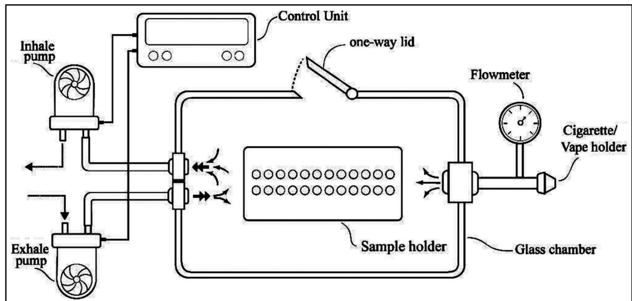
Fig.1: Smoke chamber designed and used for specimen exposure to electronic nicotine delivery system (ENDS) aerosol and cigarette smoke.
