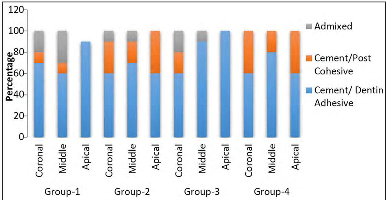
Fig.1: Percentage of modes of failure in each group.
